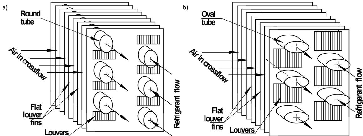
Fig. 2. Extended plain fin surfaces of interrupted geometry with multilouver fins: a) fins on round tubes; b) fins on oval (elliptic) tubes
