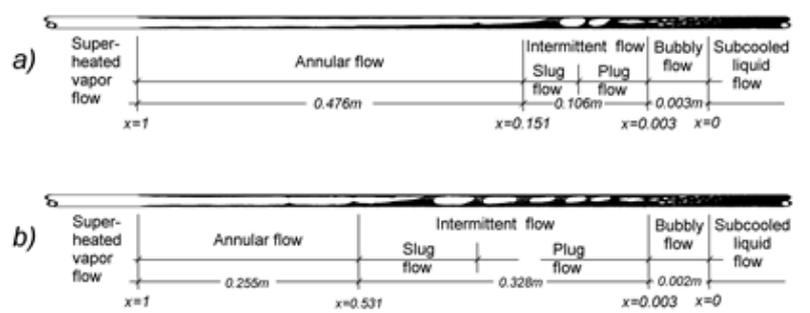
Fig. 9. Two phase flow regimes for the condenser under study determined based on (note: length and  $x$  scales are not preserved):
