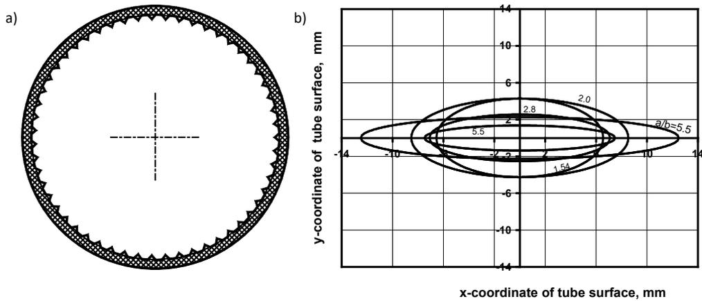
Fig. 4. Exemplary profiles of round and oval tubes applied with plain and lower fins: a) crosssection of a round tube with internal microfins (magnification  $\sim 3x$ ); b) oval tube profiles ( $a/b = \text{longer semiaxis/shorter semiaxis}$ )
