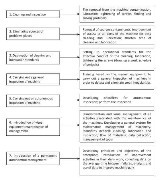
Fig. 3. Phases of Autonomous Maintenance Source: study based on (The Productivity ..., 2012, p. 65).
